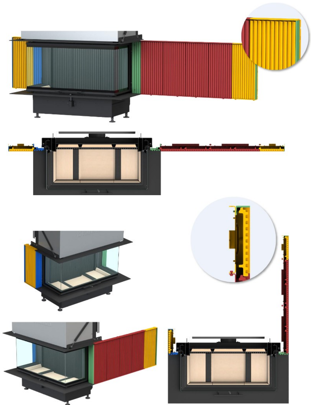
... detail (schematic) "Start-left" (blue), "Start-right" (green), "1-piece" (yellow) and "2-piece" (red) modules
